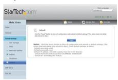
The Default window is now displayed. From the Default Window you can remotely restore the NAS Enclosure to its default settings (reset) through the web interface.
